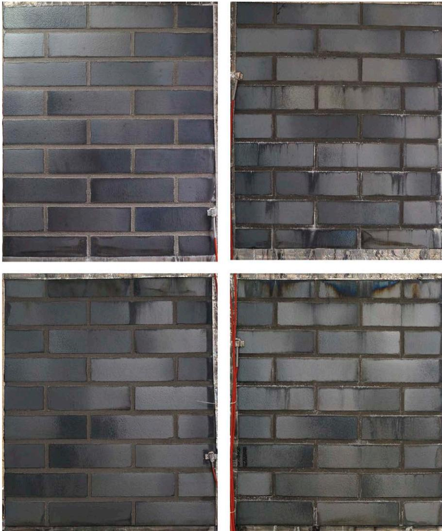
Fig. 3. Facade cladding after the weathering: S-FM joint mortar with SECON technology (left-hand half of the wall) and standard joint mortar (right-hand half of the wall), substrate of epoxy resin mortar (upper half) and bonding and reinforcement mortar (lower half) [5]
